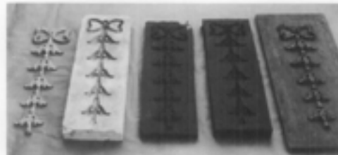
Illus. 10. The use of substitute materials is not necessarily cheaper or easier than using the original materials. The complex process of fabricating the polyester bronze reproduction pieces of the gilded wood molding for the clockcase at Independence Hall required talented artisans and substantial mold-making time. From left to right is the final molded polyester bronze detail; the plaster casting mold; the positive and negative interim neoprene rubber molds; and the expertly carved wooden master. Photo: Courtesy of Independence National Historical Park.
